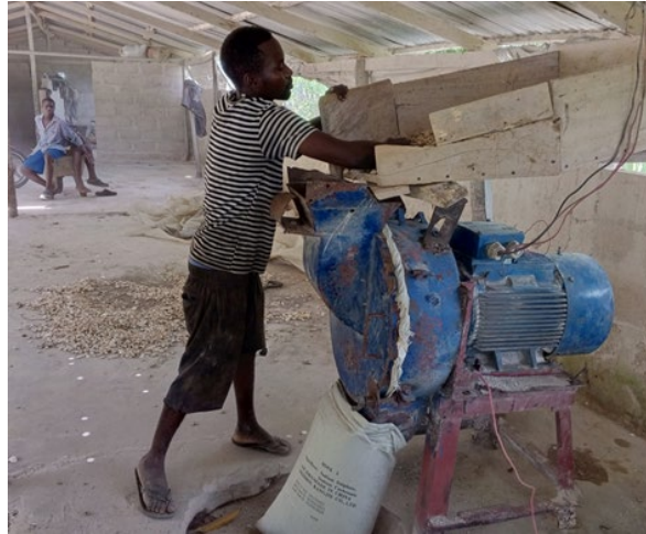
Figure 4: Shell crushing machine operated by a worker.
