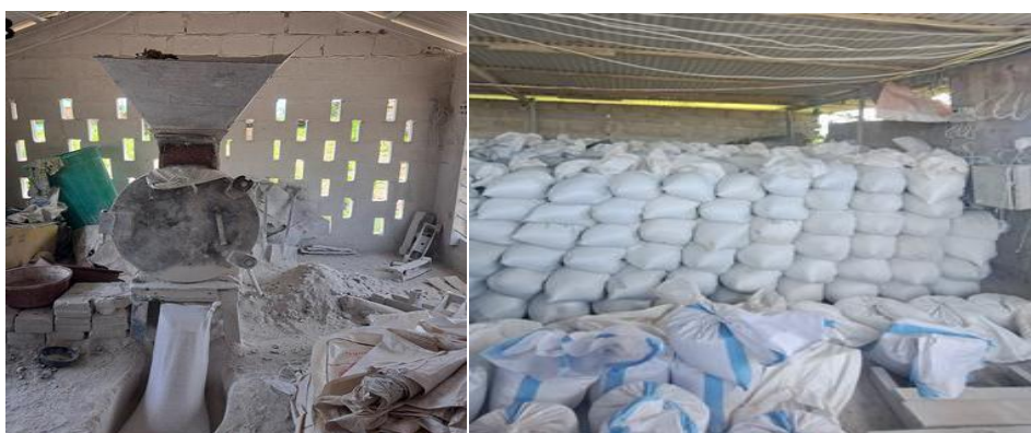
Figure 11: A shell milling machine (left) and bagged milled shell product (right).
