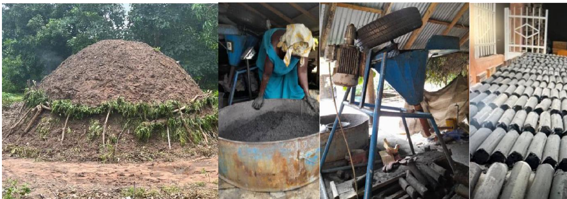
Figure 9: Traditional charcoal making from tree trunks in Bullock (left). Briquette making from leaves and other fibrous waste observed during the Senegal study tour (middle and right).
