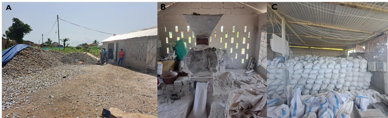
Figure 12: Shots of (A) pile of clam shells for milling, (B) shell milling machine, and (C) bagged milled shell product.
